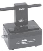
tenna has a built-in fixed battery. This battery is rechargeable via the built-in solar cell, the supplied AC adapter or via a computer USB cable. Output is to a junction cable that, in turn, has output to a 3.5mm mini plug. (Please note the BNC jack is strictly to the junction cable). This antenna is designed for indoor use only.
